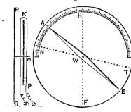
When a motionless magnetic needle is free to turn in any direction, and an electrical current is sent along a wire placed parallel to but not touching the needle, the needle has a tendency to place it-
